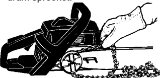
Place chain onto the sprocket
